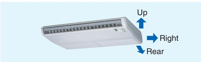
The refrigerant pipe from the unit can be arranged in three directions, rear, right and up. The drain pipe can be arranged in two directions, left and right. This will allow a free layout of piping for various installation conditions. The unit can only be serviced from the bottom.
